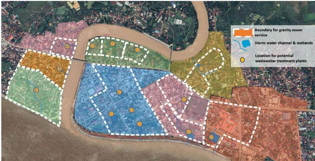
**Figure 8.2.** Mapping of the selected clusters (white line) that can be served by a gravity sewer system and possible locations for the installation of WWTPs with the effluent discharge option (yellow points) into stormwater channels and/or wetlands (blue).
