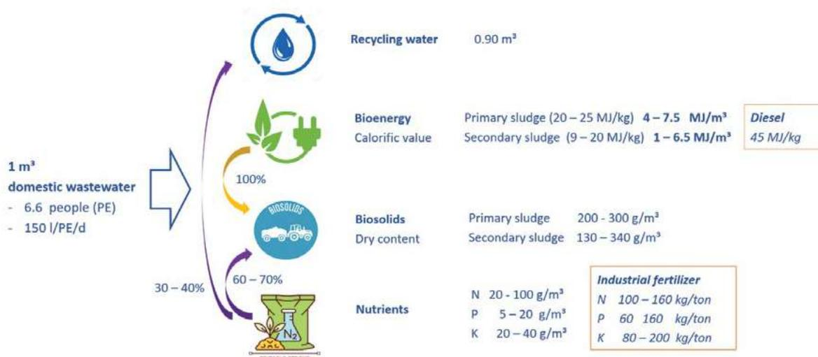
**Figure 6.2.** Potential resources that can be extracted from domestic wastewater (Source: UrbanWaters Consulting GmbH)
