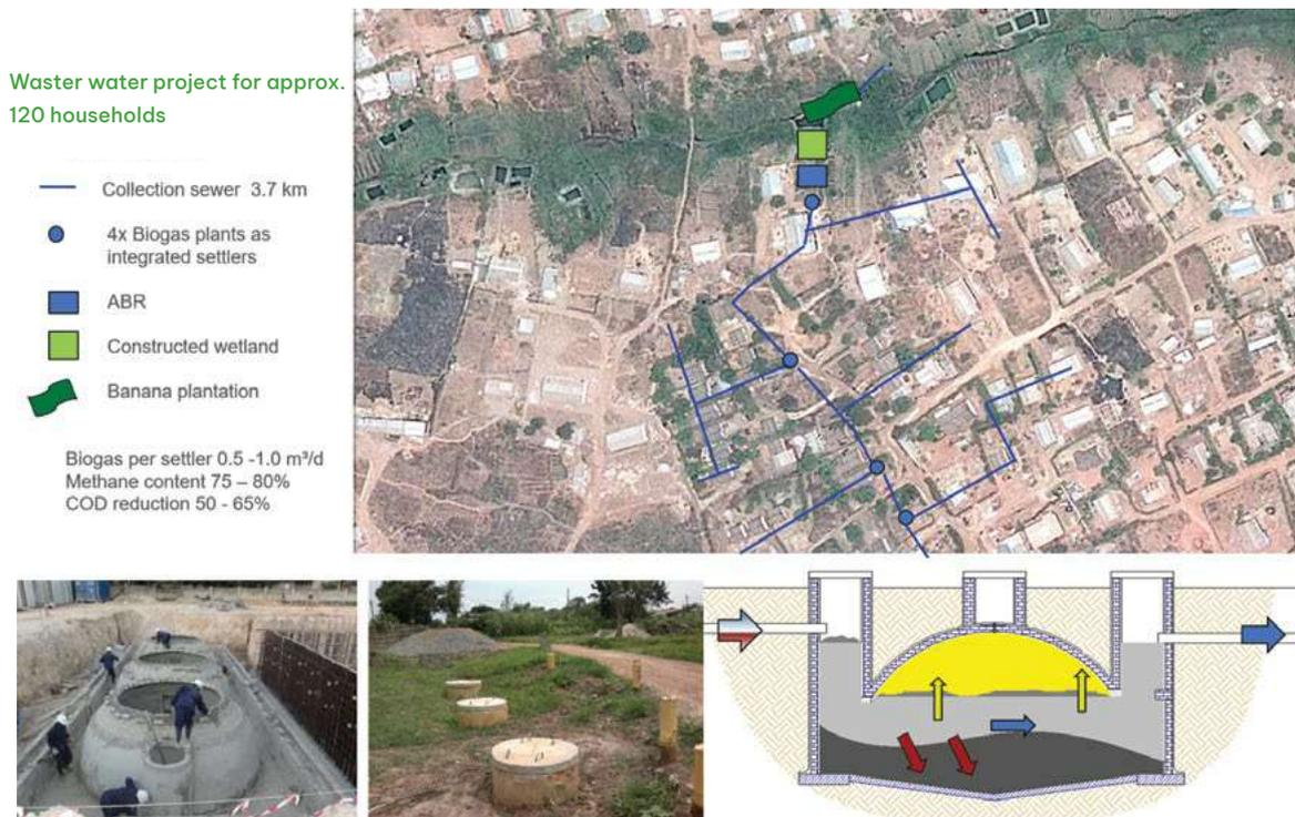
**Figure 4.7.** A project in Zambia integrated biogas settler into a sewer network
